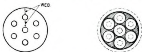
FIG. 6. Web and slivers of propellant powder grains. (Dotted lines show original grain size.)
