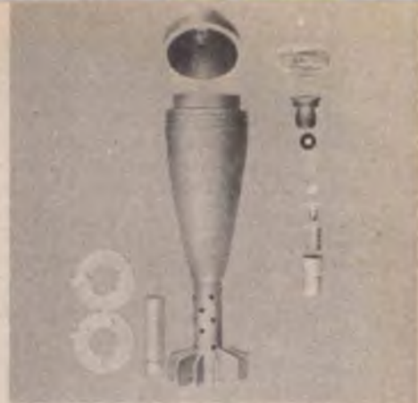
The German 'bouncing bomb', the Wurfgranate 39
