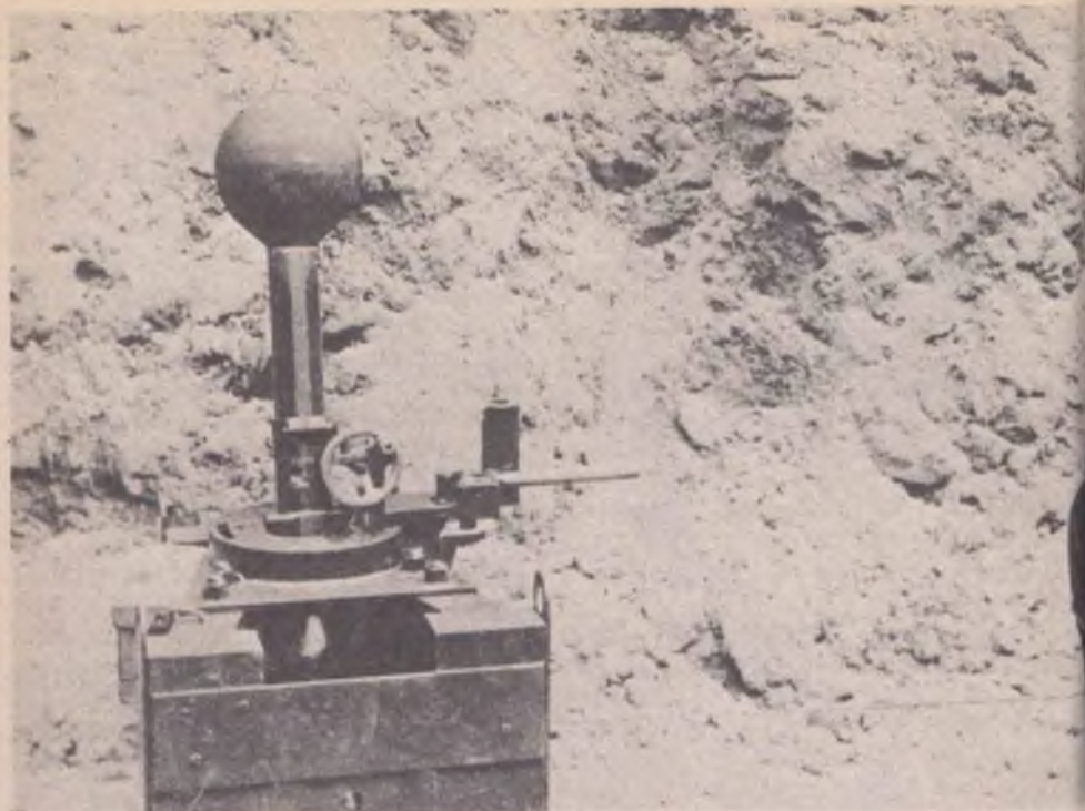
Very similar in principle to the Krupp Trench Howitzer, the Vickers 40 mm achieved a greater range by using a lighter weight bomb
