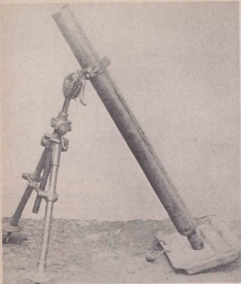
The original model 3-inch Stokes mortar approved for service in 1915
