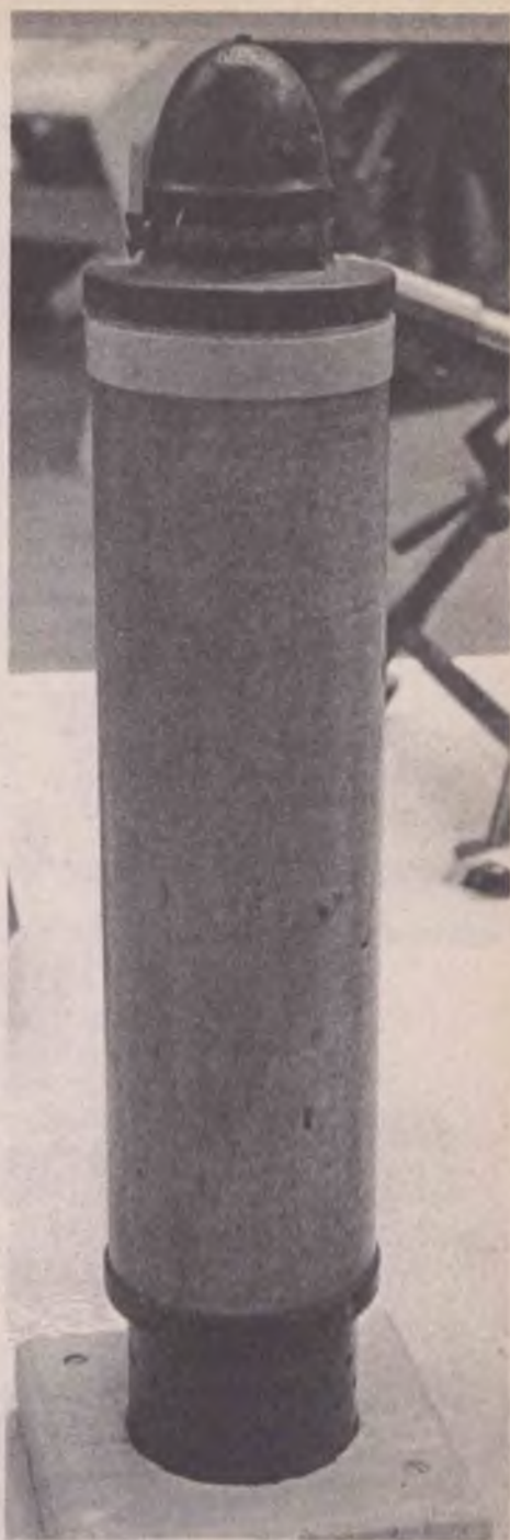
4-inch Stokes mortar bomb, generally used to send gas into the German trenches
