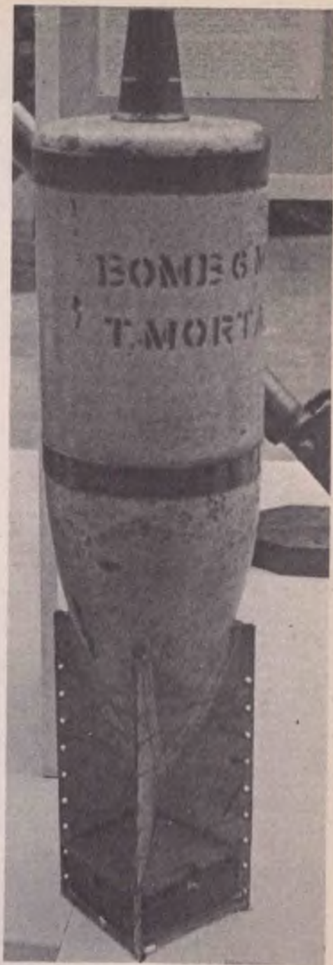
The 48-lb finned bomb fired by the 6-inch mortar. The projection on the nose of the bomb is the 'Newton' fuze
